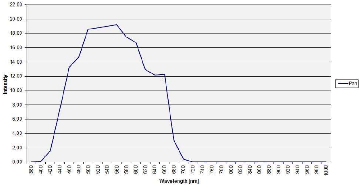
Spectral Sensitivity Vexcel UCX - Panchromatic with AR-106 Coating
