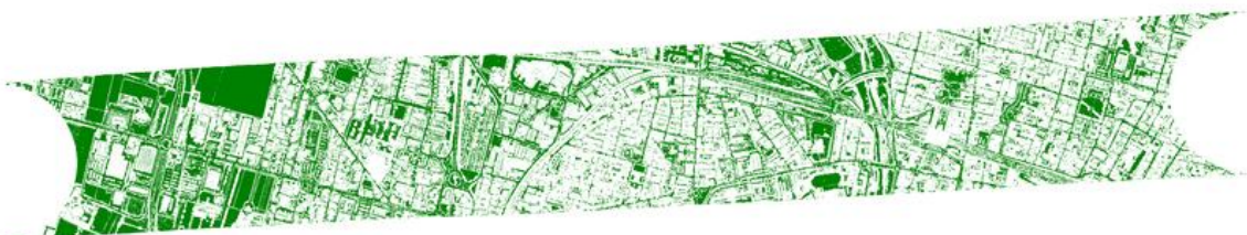
Figure 2 Vertical difference between forward and backward scan at 1000 m AGL.
